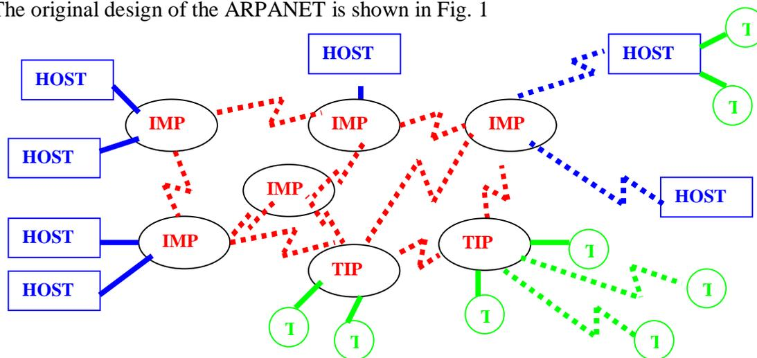
**Figure 1. Schematic of ARPANET Technology**
