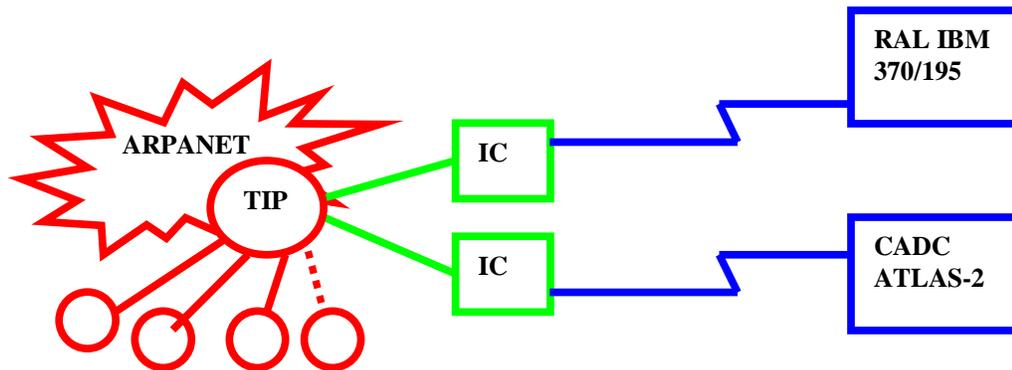
**Figure 4 Schematic of UCL methods for interfacing Hosts**
