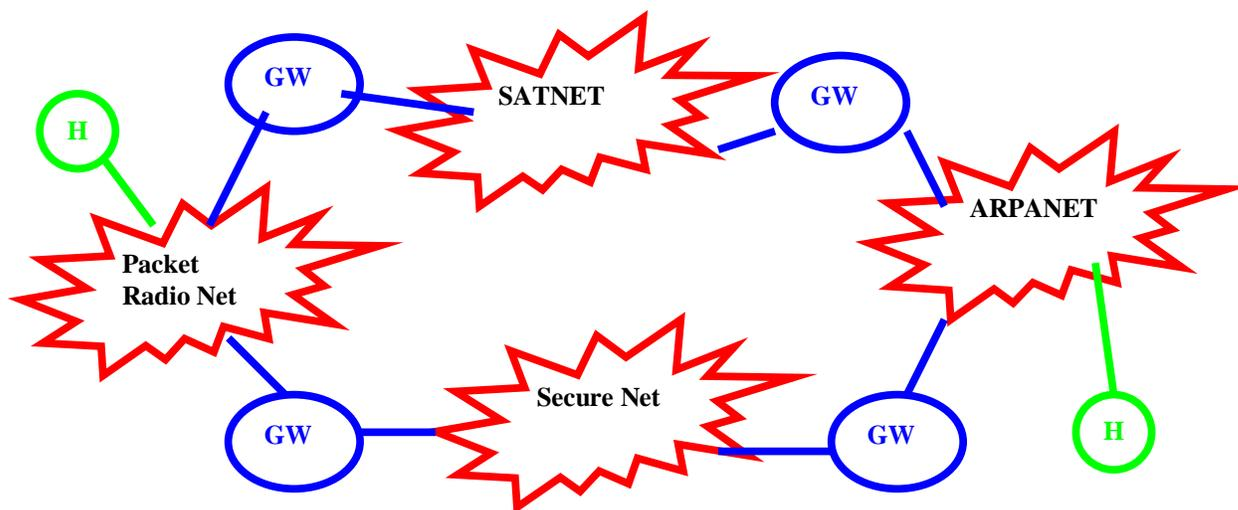
Figure 5 Connection of different Networks by Gateways
